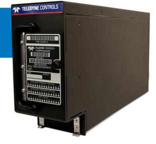
The RTMU acquires and monitors the aircraft parameters. It can
