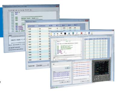
With the ACMS Tester, operators can compose and run scenario files to simulate events, trigger reports, and generate recording files. They can also send uplink commands and navigate through MCDU screens via a user-friendly, Windows-based interface that can create the equivalent of a full ACMS lab test station.
