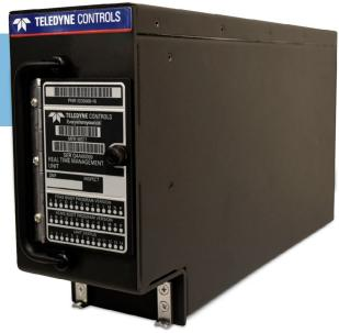
The RTMU acquires and monitors the aircraft parameters. It can generate and downlink reports via ACARS in real-time to notify the airline operator and/or the aircraft manufacturer when parameters are outside of the norm. The operator/manufacturer can then take the appropriate action in a timely manner, to support the operational safety and efficiency of the aircraft.
