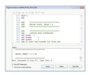
The Flight Simulation tool simulates flight profiles by replicating ARINC 429 Digital Information Transfer System (DITS) parameters. It orchestrates the emulation of the hardware complement in real-time, schedules parameter updates, and carries out operator requests and queries.
